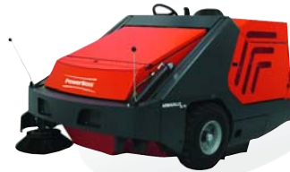
Armadillo Elite Rider Sweeper 184,800 sq.ft. per hr (17,168 sq.m.) 72" Sweeping Path* 22 cu. ft. High-Dump Hopper Gasoline, Diesel or LP Powered *Optional Left-Hand Side Broom Available
