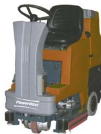
Admiral 26 Rider Scrubber 31,680 Actual sq.ft. per hr (3,188 sq. m.) 26" Scrubbing Path (66cm) 27 Gal Solution/Recovery Tank (102L) Disc or Cylindrical Brush Deck Battery Powered
