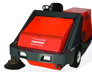
Armadillo 9XR Rider Sweeper 184,800 sq.ft. per hr (17,168 sq.m.) 72" Sweeping Path* 22 cu. ft. High-Dump Hopper Gasoline, Diesel or LP Powered *Optional Left-Hand Side Broom Available
