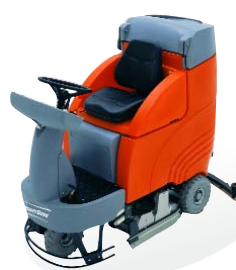
Admiral 28 & 30 Rider Scrubber 41,332 Actual sq.ft. per hr (3,840 sq. m.) 28" & 30" Scrubbing Paths (71/76cm) 30 Gal Solution/Recovery Tanks (116L) Disc or Cylindrical Brush Deck Battery Powered
